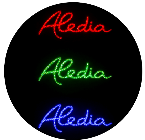
R,G, B logo light up for AR microdisplays from 200 mm wafer
